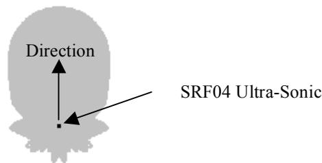
**Figure 1.** Beam Pattern for the Ultra-Sonic Ranger
